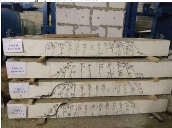
Fig. 5. Experienced beams after testing.
