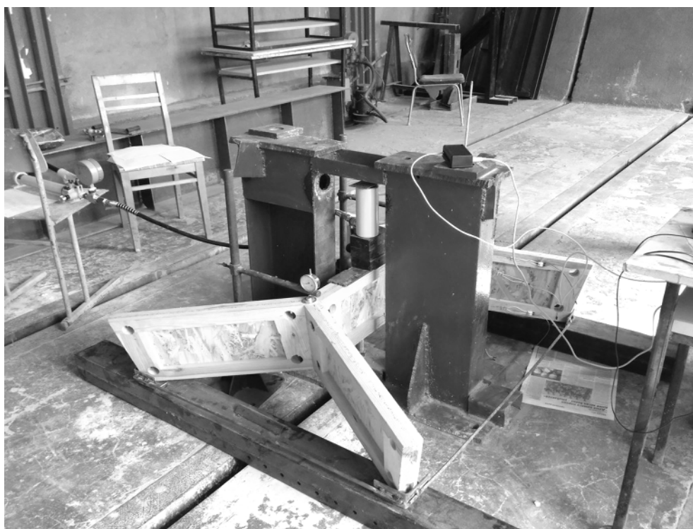
Fig. 1. A fragment of the dome under load
