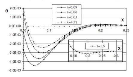
$\alpha = \alpha_1 + \alpha_2 \nu$  is the heat transfer coefficient for the medium velocity equal to  $\upsilon$ ; a is the thermal diffusivity of the body. The results of the calculations are shown in figure for the dimensionless time  $\tau = 0.03 \div 0.09$ . The calculation taking into account the temperature dependence of the thermal conductivity is performed for time  $\tau = 0.06$ .
