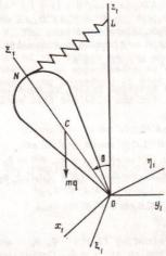
As an example of a restoring torque which depends on the angle of nutation, let us consider a rigid body with a spring attached to it at a point N, with the end L of the spring fixed (see the figure). The forces acting on the body are the force of gravity mg and the elastic force F of the spring, whose modulus is proportional to the deformation of the spring  $F = v \ (s - s_0)$ , where v is the stiffness of the spring. In this case the restoring torque
