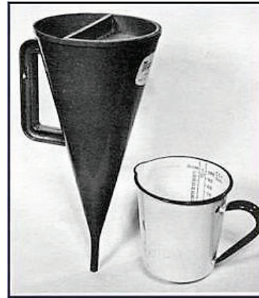
Figure 7 Viscometer "Marsh Funnel"
