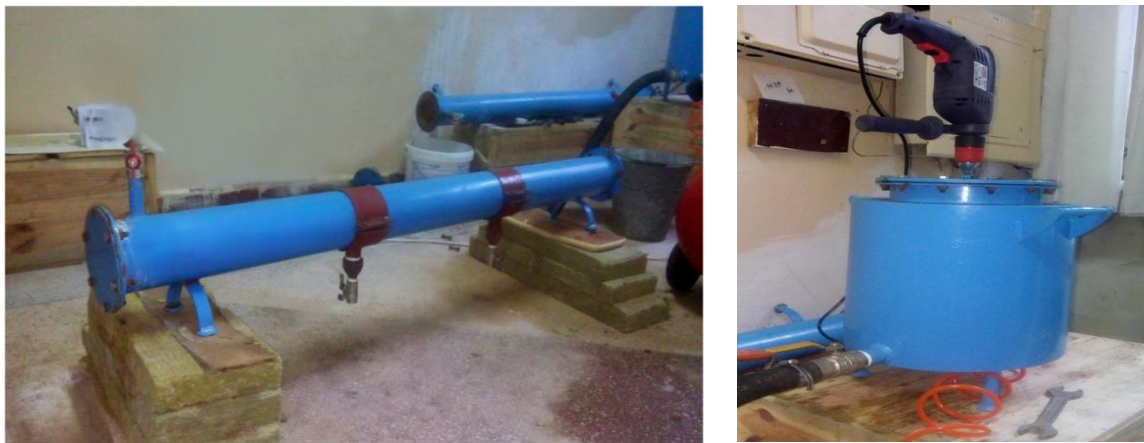
Figure 6 Laboratory test bench and mortar pumping machine
