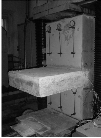
Figure 3. The general view of test sample, that is mounted on press platform
