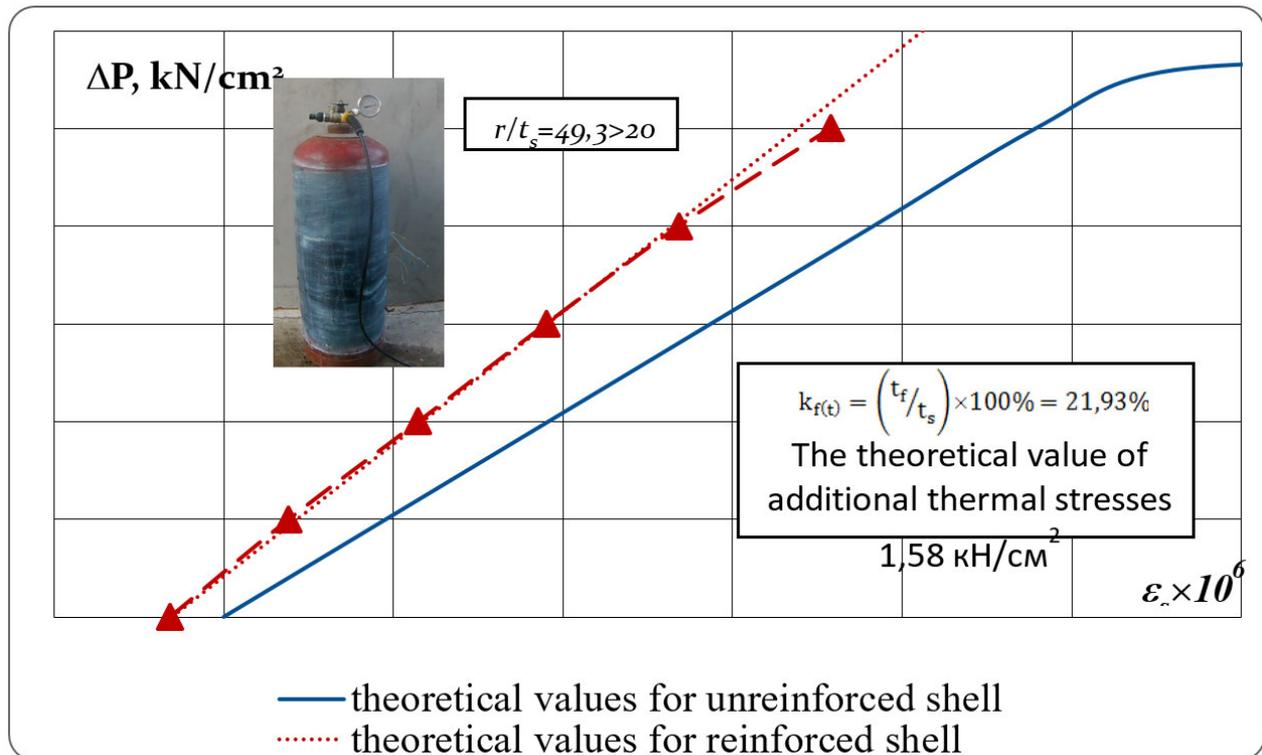
Fig. 11. The dependences of the ring strains  $\varepsilon_s$  on the internal pressure  $\Delta P$ , obtained with a change in operating temperature by  $+24^\circ\text{C}$  in a steel cylindrical shell with an inner diameter of  $299.0 \pm 0.1$  mm and a wall thickness of  $3.0 \pm 0.1$  mm, reinforced by external transverse FRP of the *MapeWrap C UNI-AX HM* system installed in 2 layers
