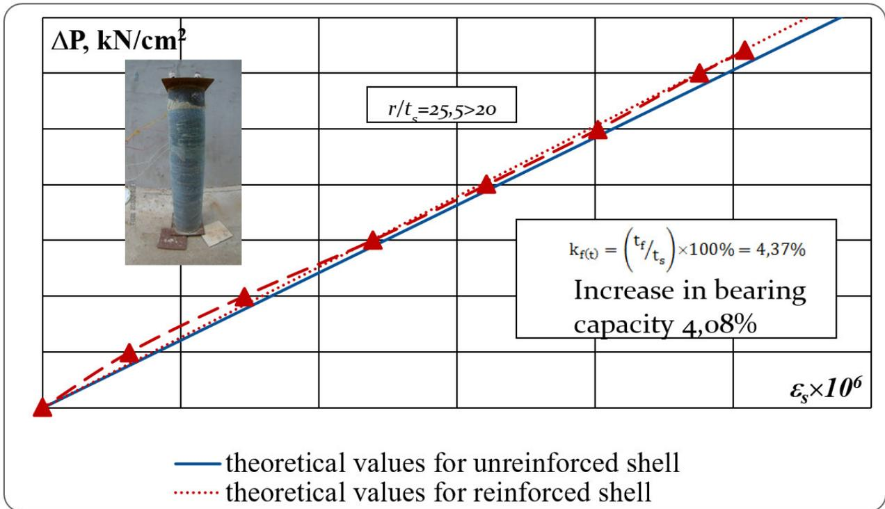
Fig. 3. The dependences of the ring strains  $\varepsilon_s$  on the internal pressure  $\Delta P$  in a steel cylindrical shell with an inner diameter of  $150.0 \pm 0.1$  mm and a wall thickness of  $3.0 \pm 0.1$  mm, reinforced by external transverse FRP of the *SikaWrap-230C* system installed in 1 layer
