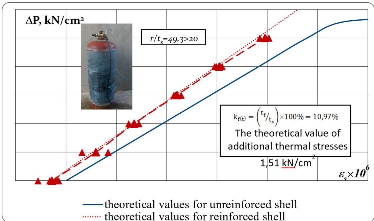
Fig. 10. The dependences of the ring strains  $\varepsilon_s$  on the internal pressure  $\Delta P$ , obtained with a change in operating temperature by  $+36^\circ\text{C}$  in a steel cylindrical shell with an inner diameter of  $299.0 \pm 0.1$  mm and a wall thickness of  $3.0 \pm 0.1$  mm, reinforced by external transverse FRP of the *MapeWrap C UNI-AX HM* system installed in 1 layer
