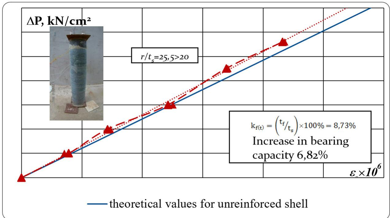
Fig. 4. The dependences of the ring strains  $\varepsilon_s$  on the internal pressure  $\Delta P$  in a steel cylindrical shell with an inner diameter of  $150.0 \pm 0.1$  mm and a wall thickness of  $3.0 \pm 0.1$  mm, reinforced by external transverse FRP of the *SikaWrap-230C* system installed in 2 layers
