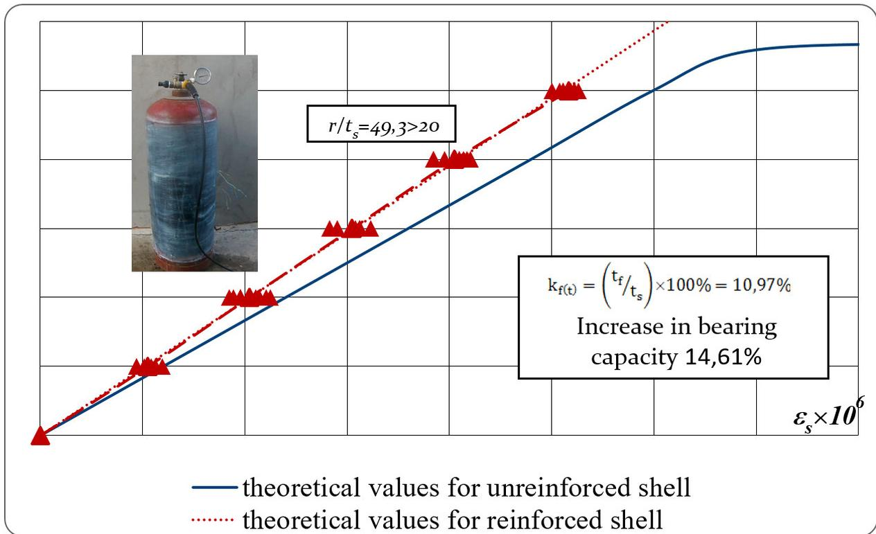
Fig. 7. The dependences of the ring strains  $\varepsilon_s$  on the internal pressure  $\Delta P$  in a steel cylindrical shell with an inner diameter of  $299.0 \pm 0.1$  mm and a wall thickness of  $3.0 \pm 0.1$  mm, reinforced by external transverse FRP of the *MapeWrap C UNI-AX HM* system installed in 1 layer
