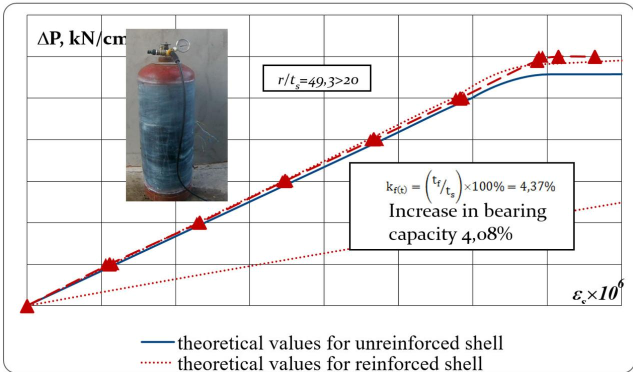
Fig. 5. The dependences of the ring strains  $\varepsilon_s$  on the internal pressure  $\Delta P$  in a steel cylindrical shell with an inner diameter of  $299.0 \pm 0.1$  mm and a wall thickness of  $3.0 \pm 0.1$  mm, reinforced by external transverse FRP of the *SikaWrap-230C* system installed in 1 layer
