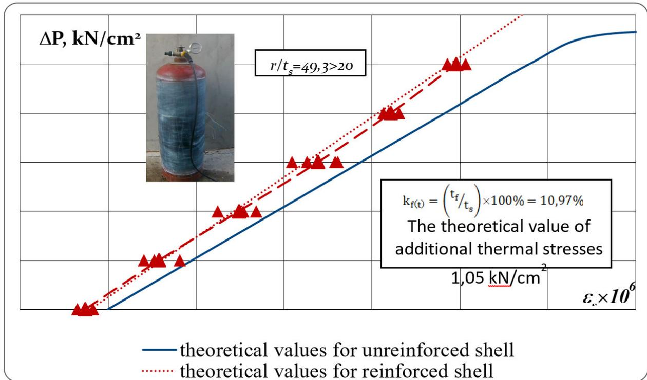
Fig. 9. The dependences of the ring strains  $\varepsilon_s$  on the internal pressure  $\Delta P$ , obtained with a change in operating temperature by  $+25^\circ\text{C}$  in a steel cylindrical shell with an inner diameter of  $299.0 \pm 0.1$  mm and a wall thickness of  $3.0 \pm 0.1$  mm, reinforced by external transverse FRP of the *MapeWrap C UNI-AX HM* system installed in 1 layer
