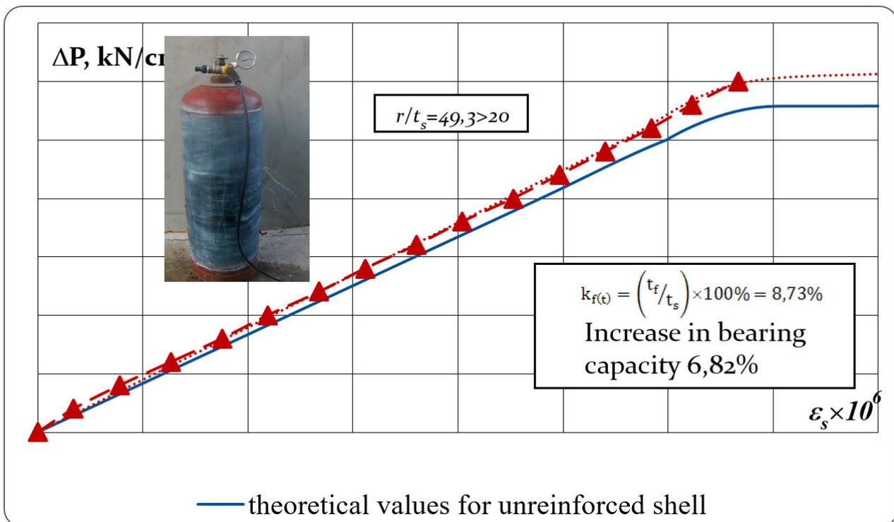
Fig. 6. The dependences of the ring strains  $\varepsilon_s$  on the internal pressure  $\Delta P$  in a steel cylindrical shell with an inner diameter of  $299.0 \pm 0.1$  mm and a wall thickness of  $3.0 \pm 0.1$  mm, reinforced by external transverse FRP of the *SikaWrap-230C* system installed in 2 layers
