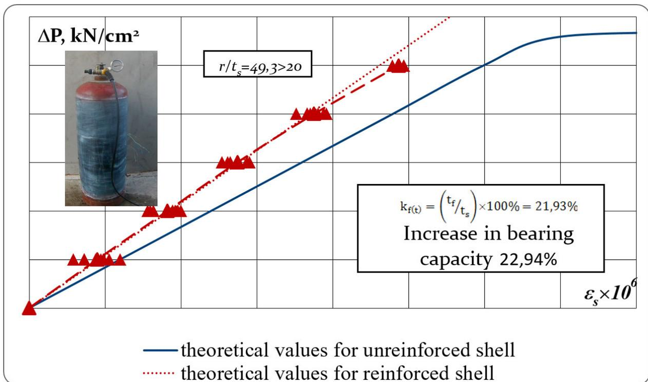
Fig. 8. The dependences of the ring strains  $\varepsilon_s$  on the internal pressure  $\Delta P$  in a steel cylindrical shell with an inner diameter of  $299.0 \pm 0.1$  mm and a wall thickness of  $3.0 \pm 0.1$  mm, reinforced by external transverse FRP of the *MapeWrap C UNI-AX HM* system installed in 2 layers
