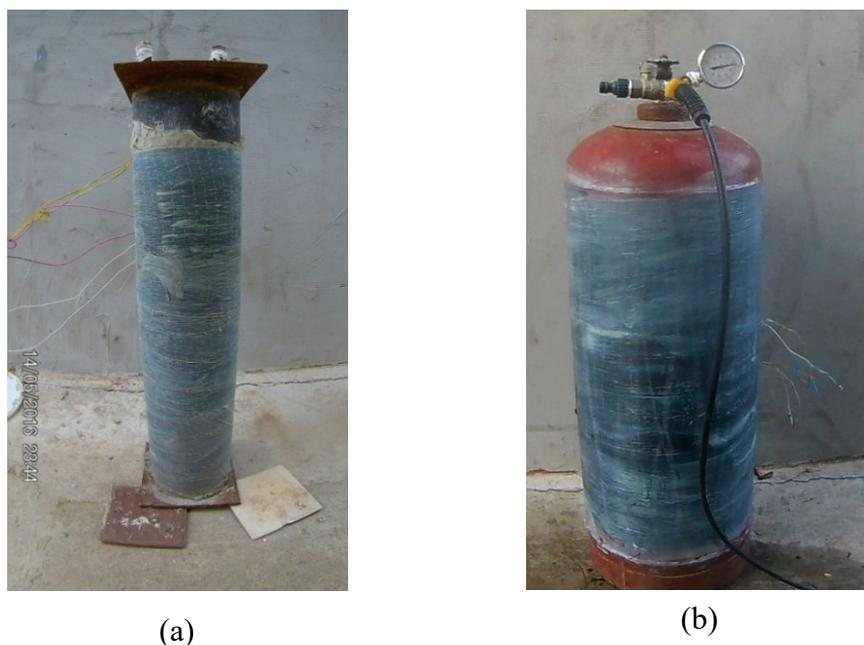
Fig. 2. Experimental samples made of: a – welded pipes with an inner diameter of  $150.0 \pm 0.1$  mm, wall thickness of  $3.0 \pm 0.1$  mm ( $r/t_s = 25 > 20$ ), b – welded steel cylinders with an outer diameter of  $299.0 \pm 0.1$  mm, wall thickness  $3.0 \pm 0.1$  mm,  $\Delta CTY ISO 10462:2019$  ( $r/t_s = 49,3 > 20$ )
