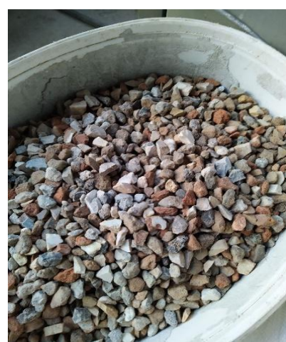
secondary crushed stone from recycled brickwork and ceramic tiles
