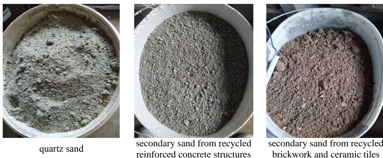
Fig. 2. Types of sand used for concrete production
