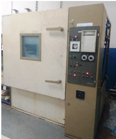
Fig. 4. Climatic chamber for testing the term of effective material use
