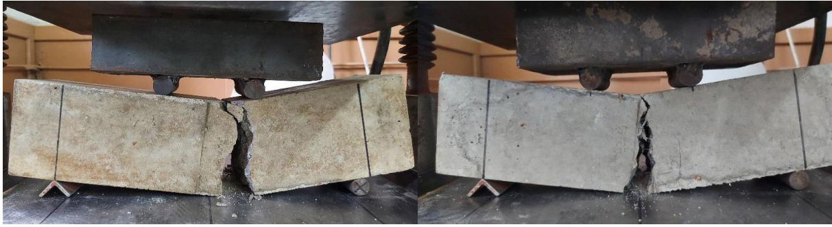
Fig. 4. The nature of the destruction of samples not modified (left) and dispersed reinforced concrete (right) after tensile bending test
