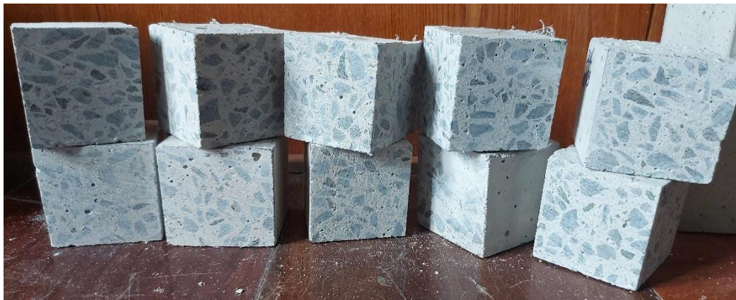
Fig. 5. Made cube samples with a rib length of 70 mm for abrasion test
