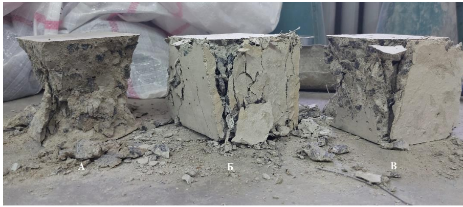
Fig. 2. The nature of the destruction of samples of classical and dispersed reinforced concrete: a – concrete without dispersed reinforcement; b – fiber concrete using fiber "Baumesh"; c – fiber concrete using steel fiber
